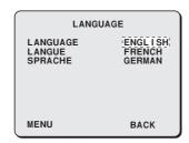
**2** Use the joystick lever (↑↓) to select the language used for display and press the [ENTER] button.
